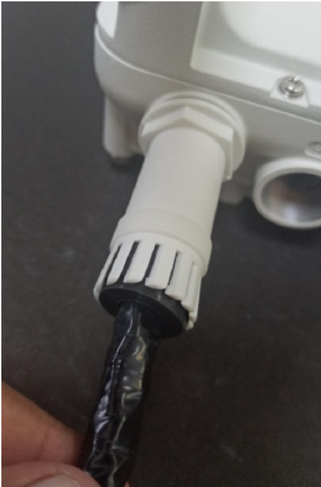
Figure 139: Fitting the gland body
