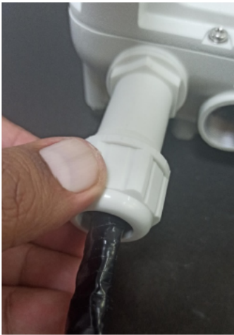
Figure 141: Fitting the gland nut to the rubber seal
