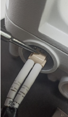
Figure 143: Pulling the bale clasp (latch)
