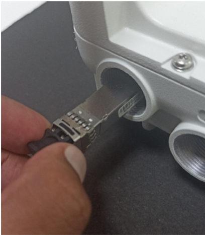
Figure 135: Pushing the module home
