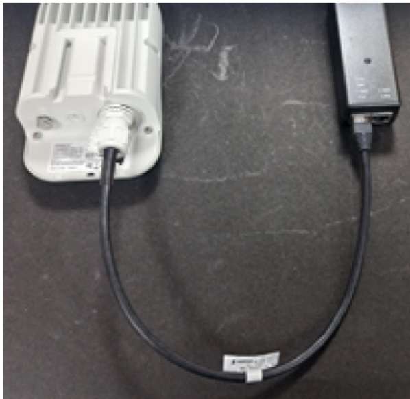
Figure 128: Connecting the V1000 power injector
