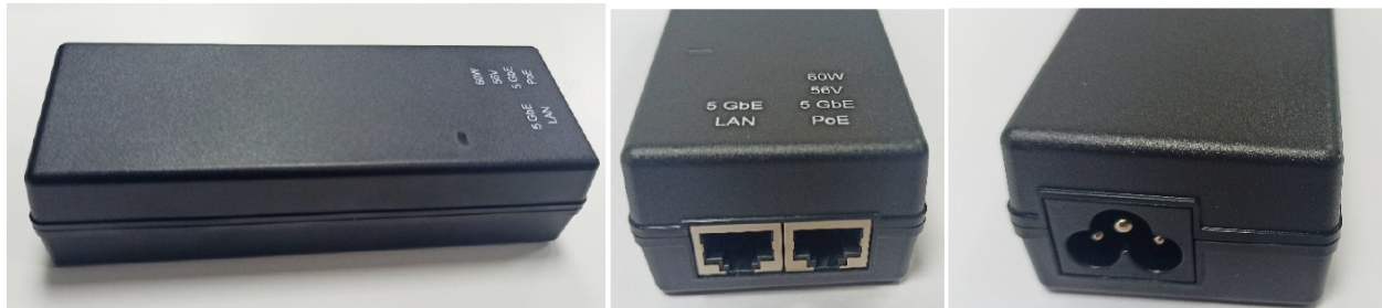
Figure 35: PoE power supply to V3000 or V5000
