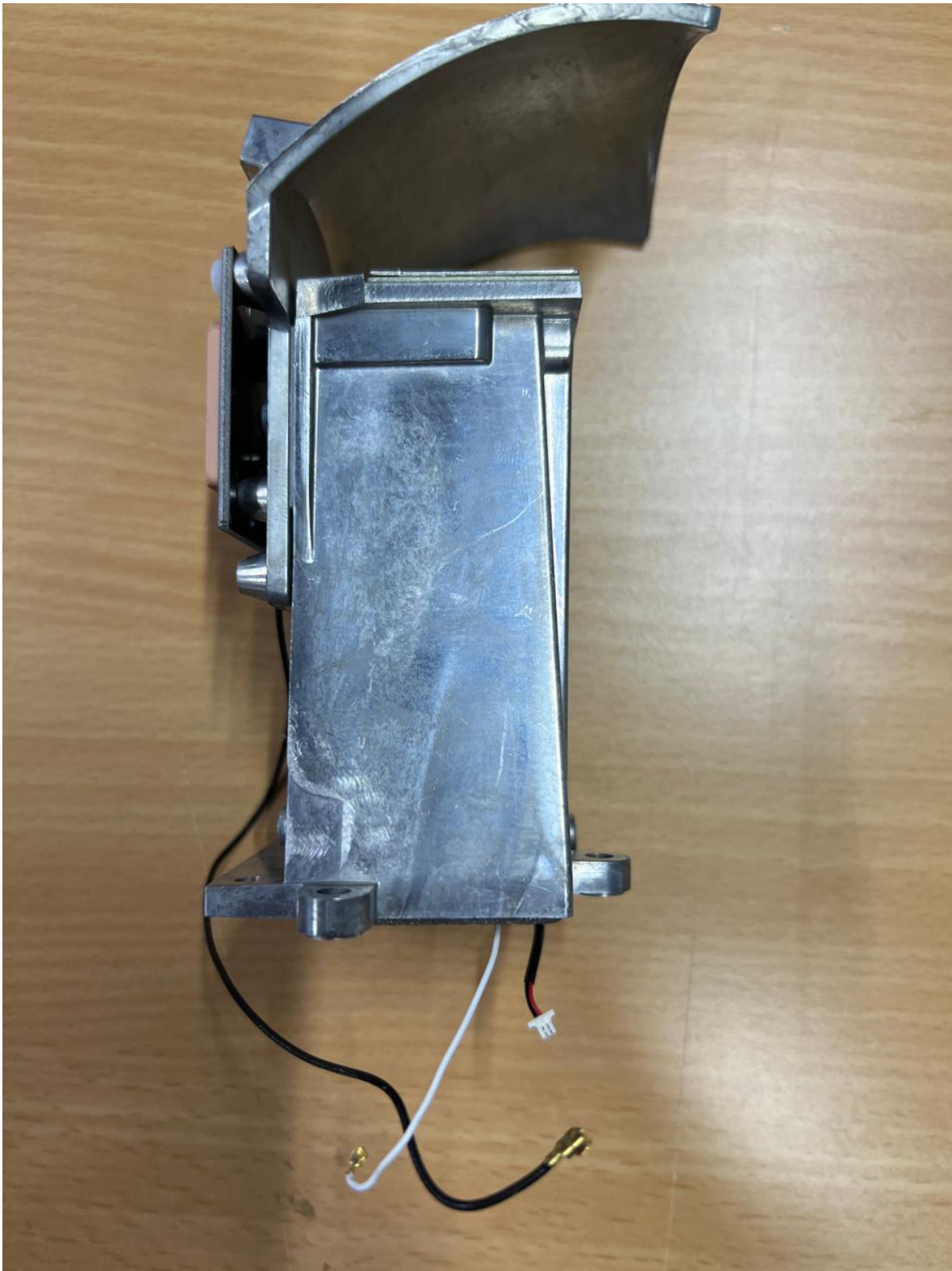
60 GHz cnWave V2000 RF Tile Holder with Sub-Reflector and RF Tile Left Hand Side View
