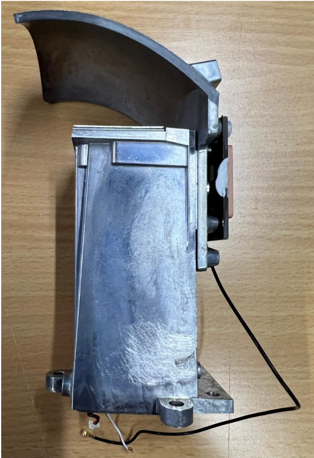
60 GHz cnWave V2000 RF Tile Holder with Sub-Reflector and RF Tile Right Hand Side View
