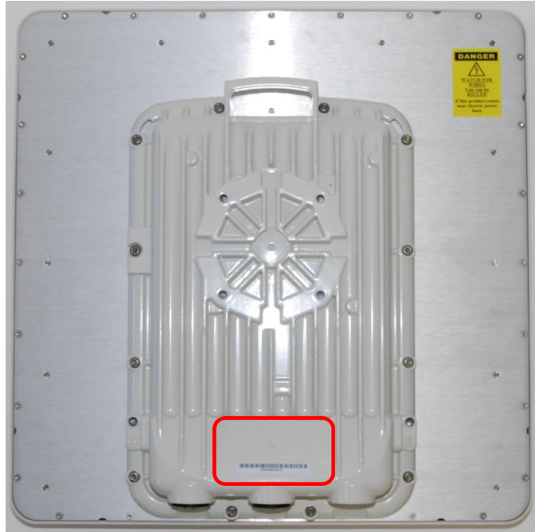
Integrated ODU Rear View with Label Position highlighted in Red
