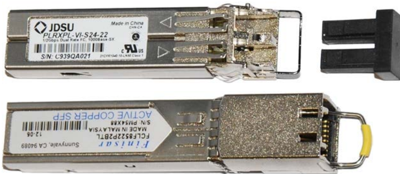
Figure 20 Optical or copper SFP transceiver module
