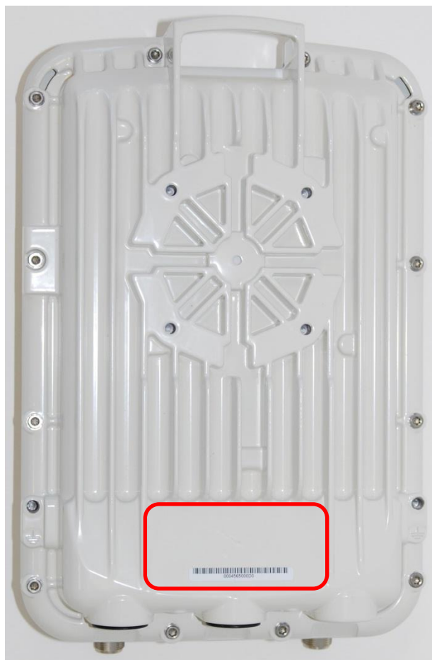
Connectorized ODU Rear View with Label Position highlighted in Red
