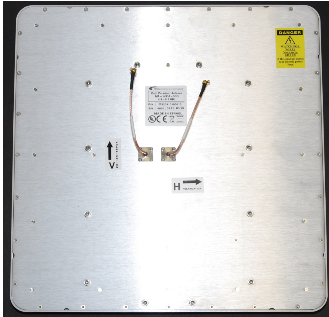
Rear of Integrated Antenna which forms the Front Cover of the ODU
