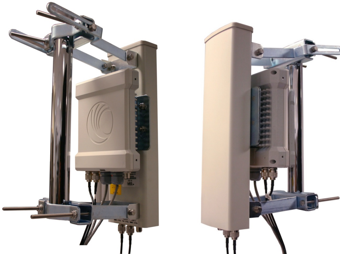
Figure 101 Mounted PMP 450 AP and antenna assembly, viewed from back and back
