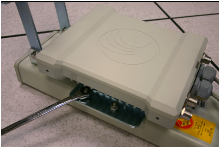
Figure 100 Lower bracket attached to AP antenna
