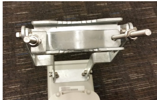
Figure 88 Assembled upper bracket connected to AP antenna
