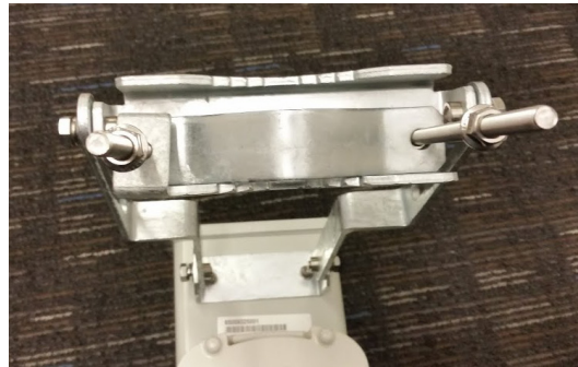
Figure 60 Assembled upper bracket connected to AP antenna
