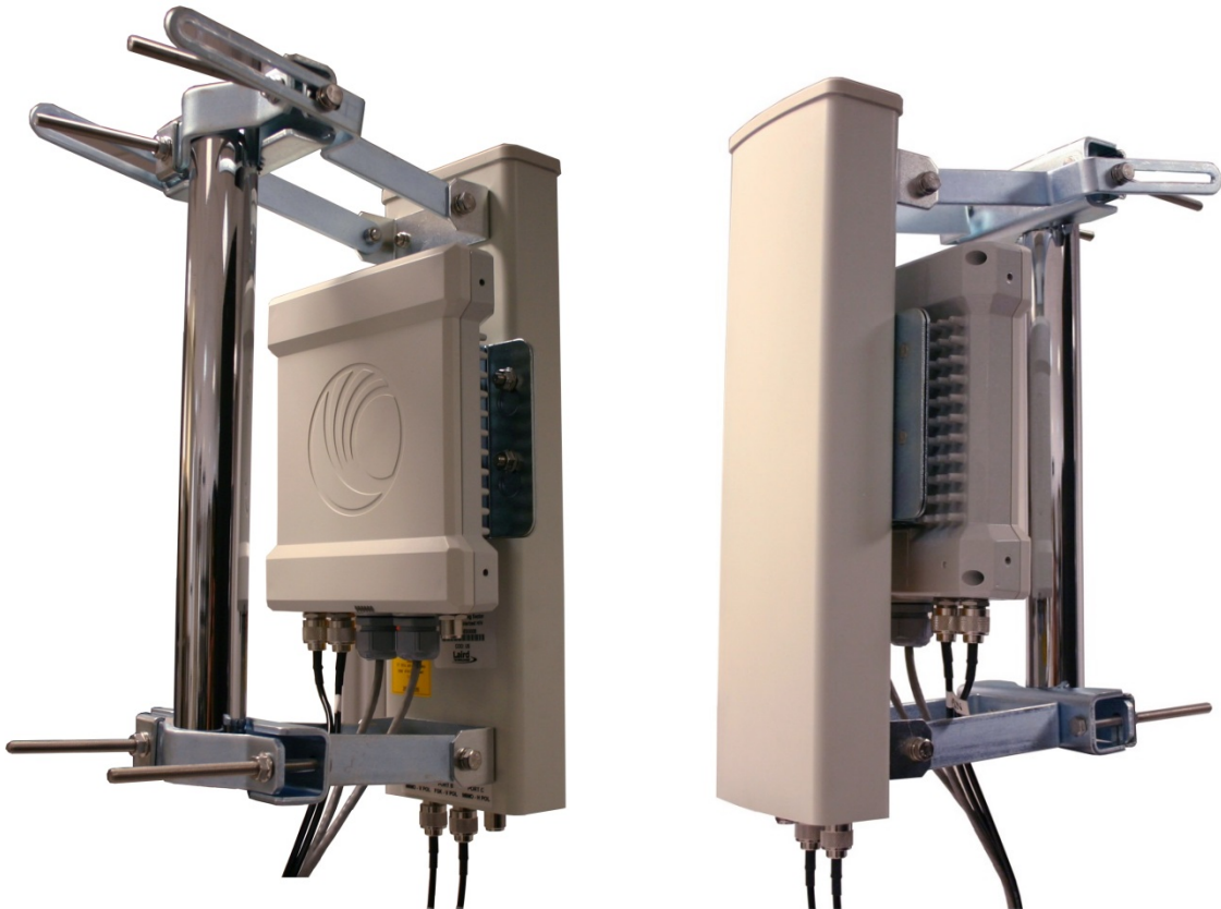
Figure 73 Mounted PMP 450 AP and antenna assembly, viewed from back and back
