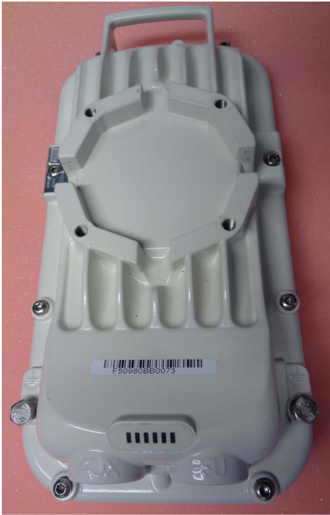
PMP 450i / PTP 450i Rear View - Connectorized ODU available as AP, SM or PTP
