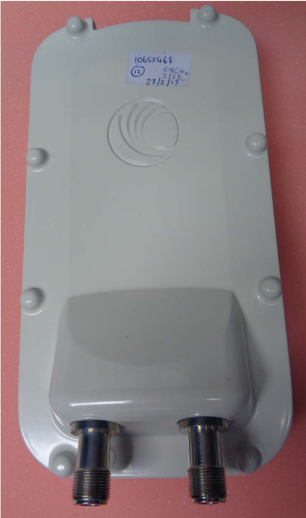
PMP 450i / PTP 450i Front View - Connectorized ODU available as AP, SM or PTP
