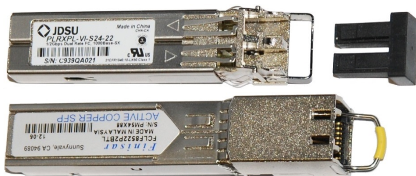
Figure 25 Optical or copper SFP transceiver module
