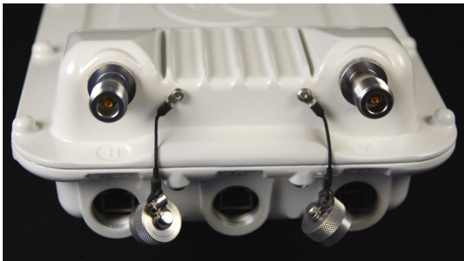
Figure 16 Connectorized ODU antenna interfaces
