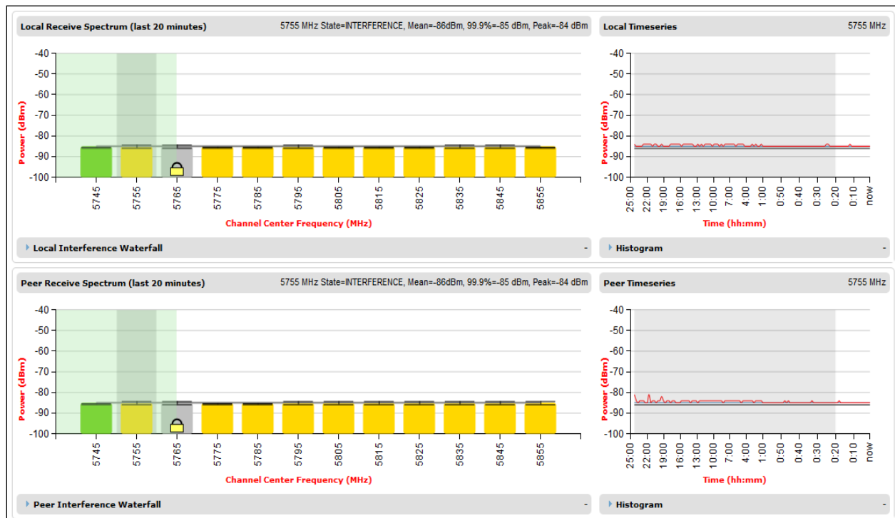
Figure 193 Spectrum Expert page with Receive Spectrum and Timeseries for both Local and Peer
