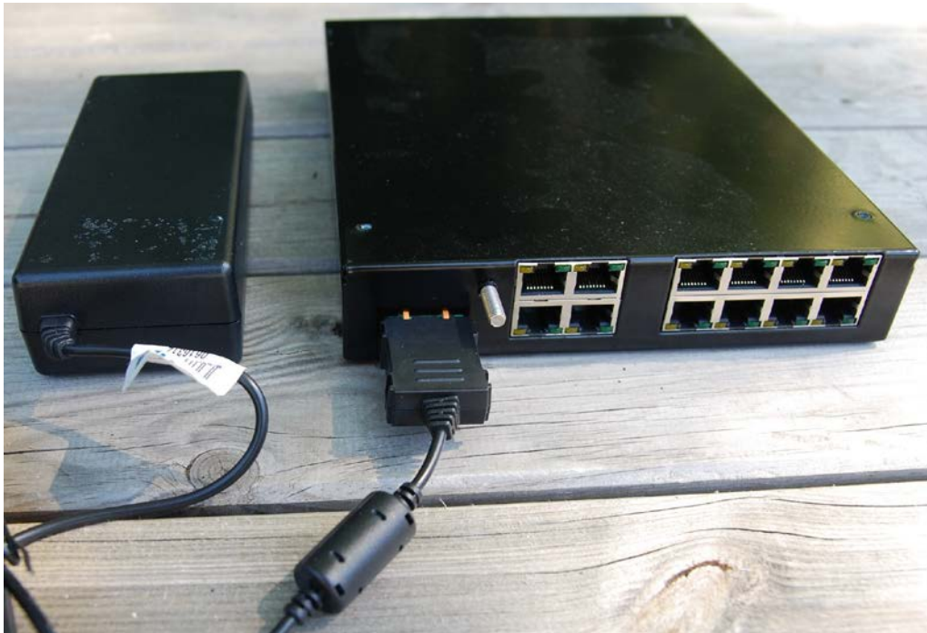
Figure 121 NIDU powered by the PTP 800 AC-DC Power Supply Converter
