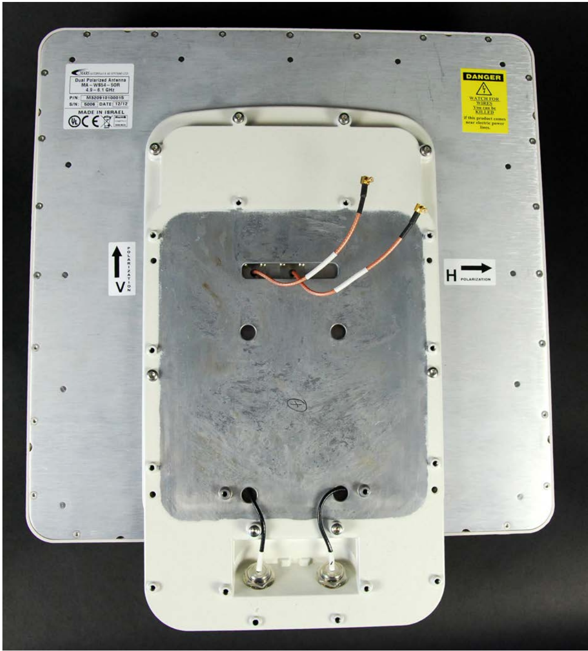
PTP 700 Rear View – Connectorized + Integrated ODU Plate fitted to Antenna
