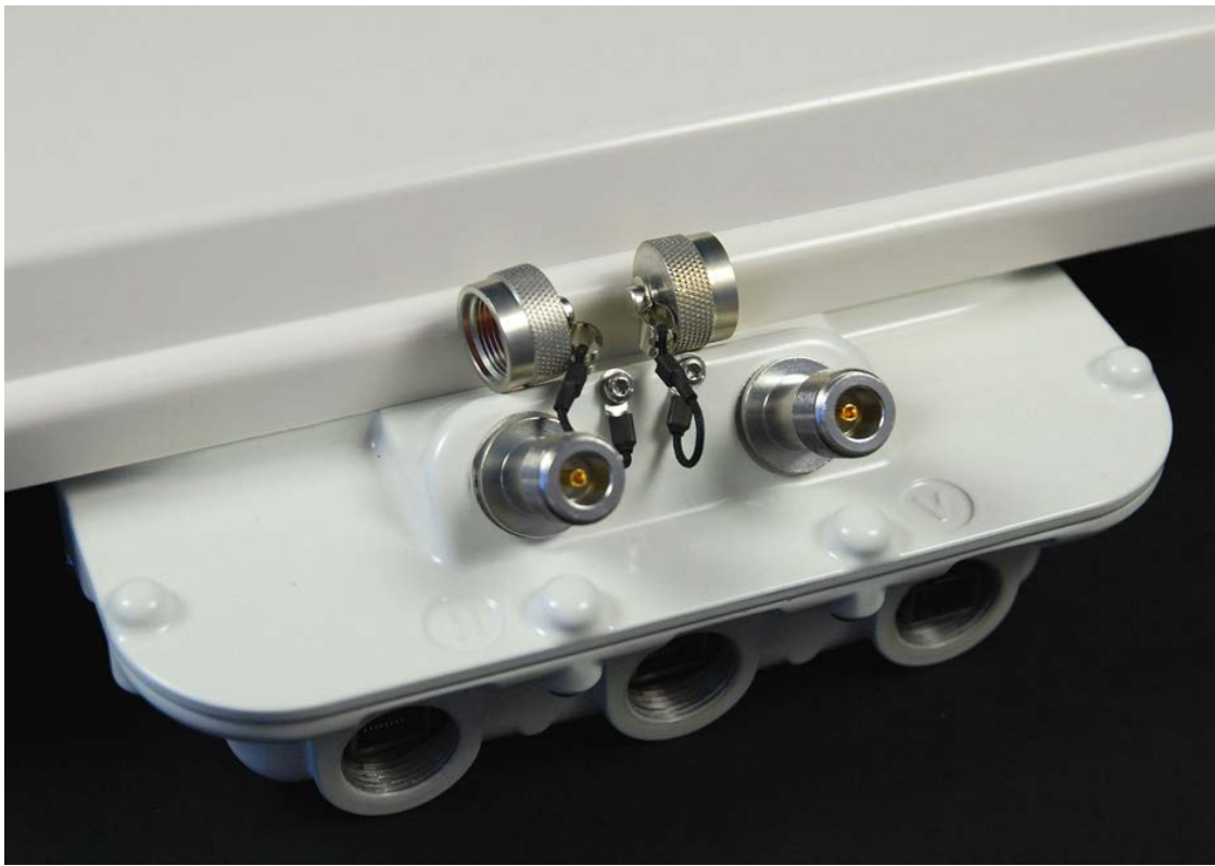
PTP 700 Connectorized + Integrated ODU - RF Connectors with Covers Removed
