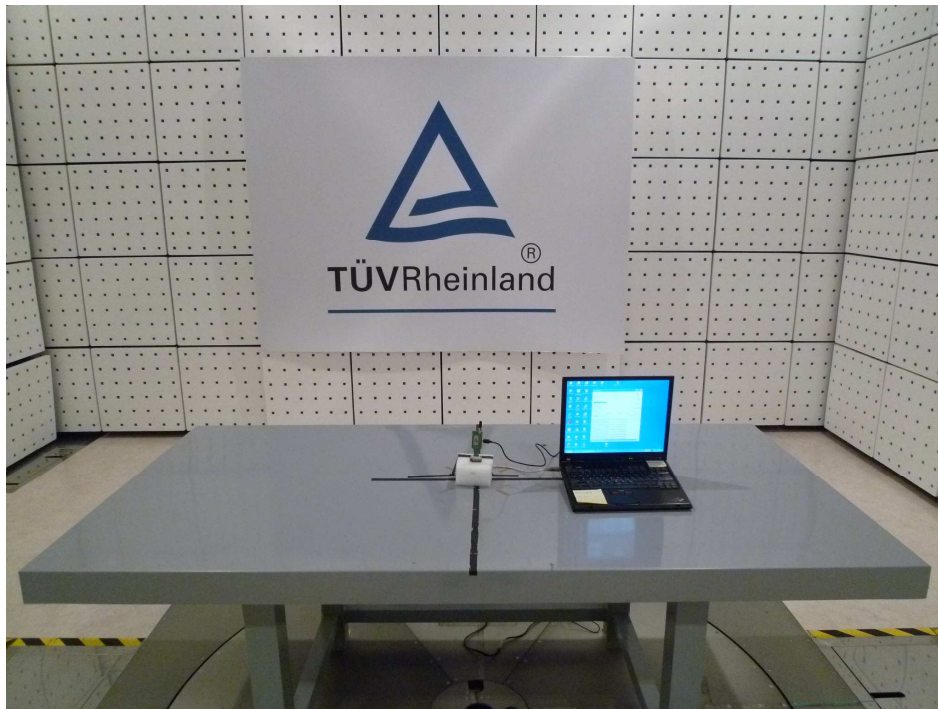
Photograph 1: Set-up for Spurious Emissions (Front View)
