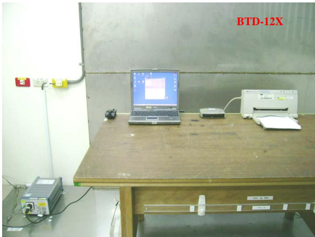
**Photo 2: Conducted Emission Test Set-up**
