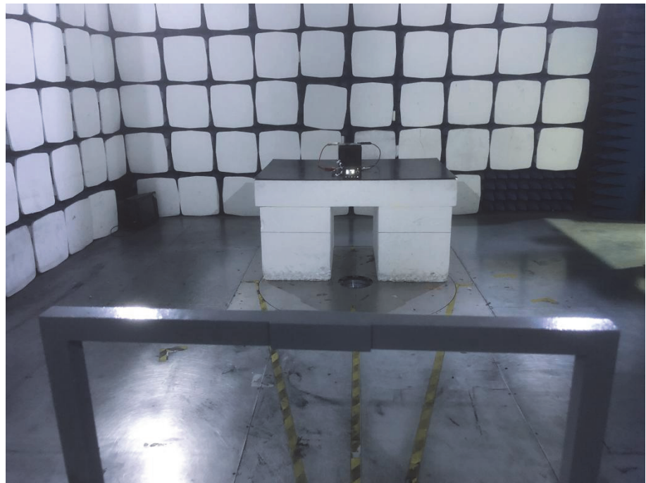
Radiation Emission Test Setup (Below 30MHz)
