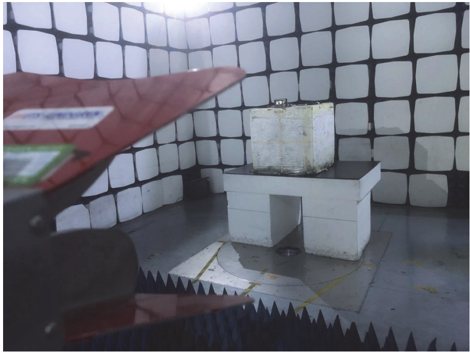
Radiation Emission Test Setup (1GHz to 18GHz)
