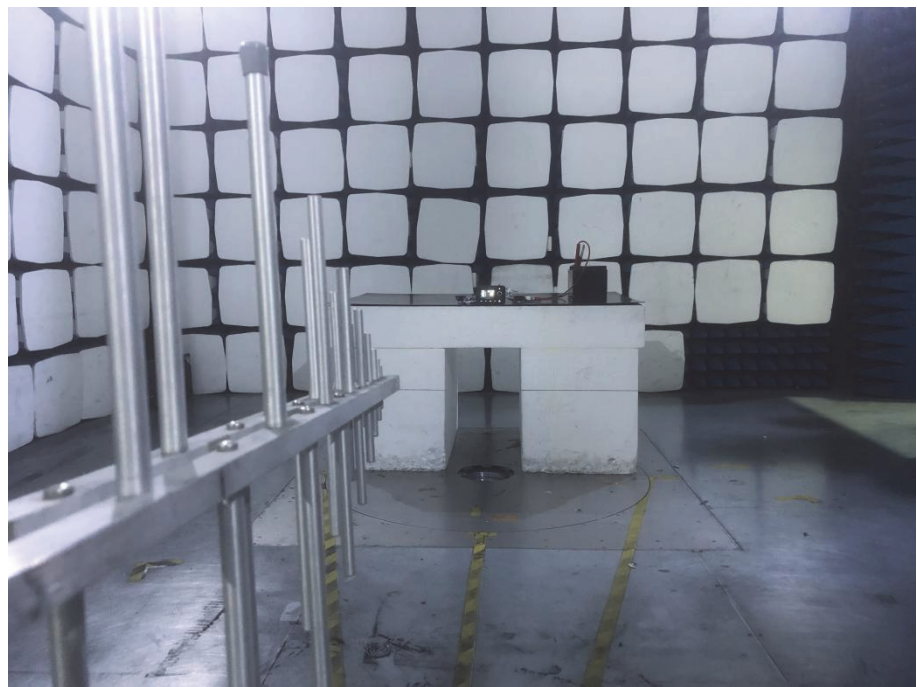
Radiation Emission Test Setup (30MHz to 1GHz)
