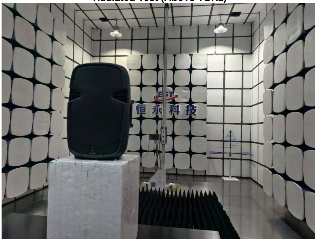
Radiated Test (Above 1GHz)
