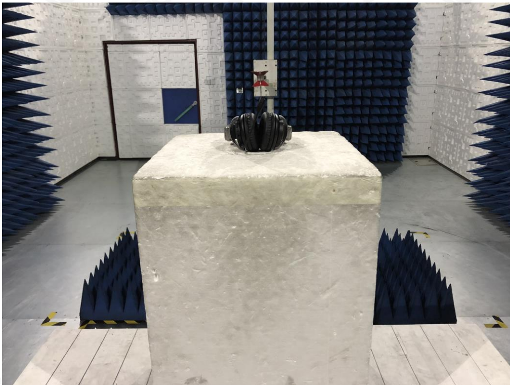
RADIATED EMISSION TEST SETUP ABOVE 1GHZ
