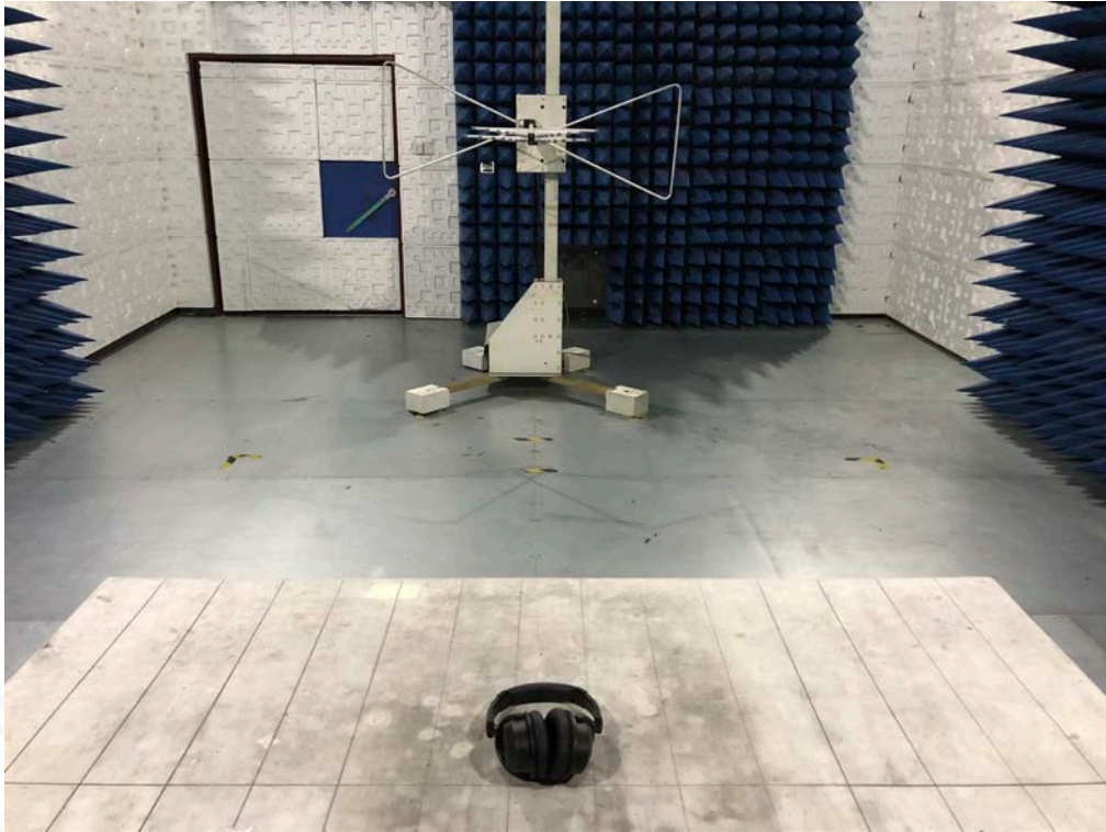
RADIATED EMISSION TEST SETUP ABOVE 1GHZ
