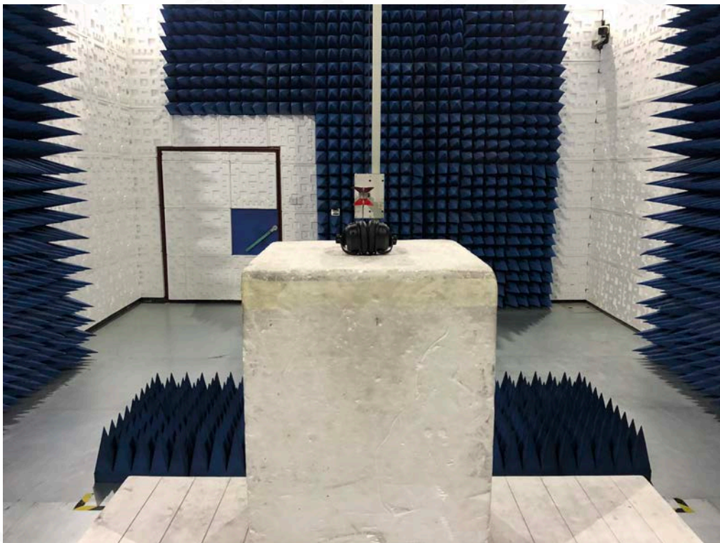
RADIATED EMISSION TEST SETUP ABOVE 1GHZ
