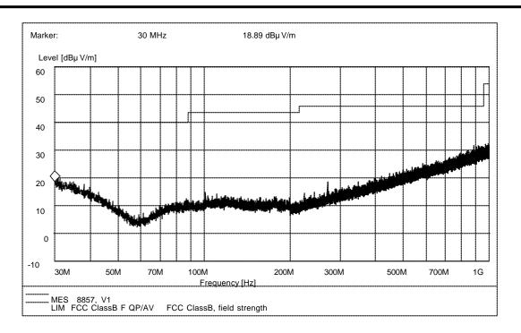
3. Radiation disturbances, maxpeak detector, 30MHz-1000MHz, antenna polarization: Horizontal
