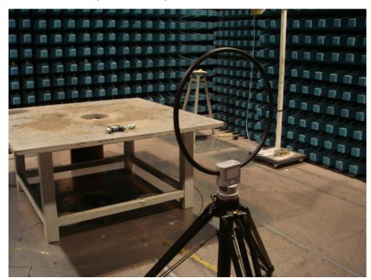
2. Radiated Emission Test (30MHz~1000MHz)
