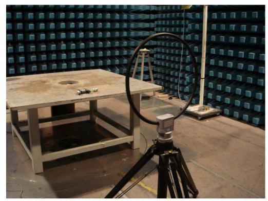
2. Radiated Emission Test (30MHz~1000MHz)
