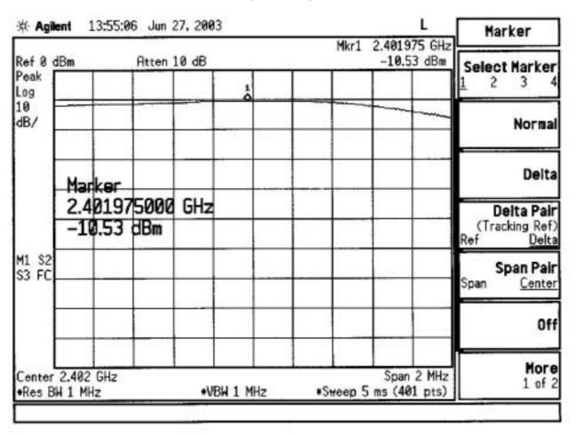
The Power (ERP) = Output power + cable loss + antenna gain = -10.53 dbm + 3.6 db+ 1 dBi = -5.93 dbm
