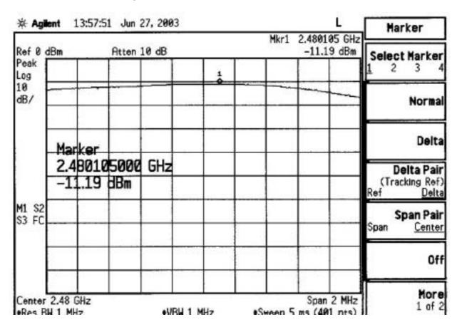
The Power (ERP) = Output power + cable loss + antenna gain
