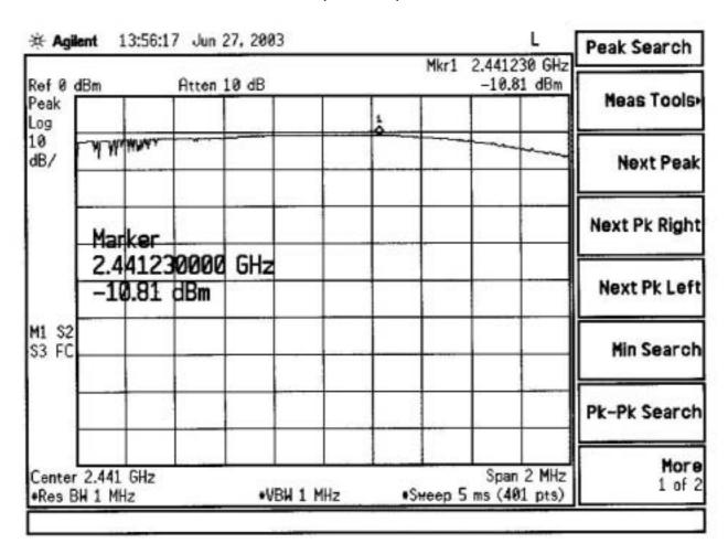
The Power (ERP) = Output power + cable loss + antenna gain = -10.81 dbm + 3.6 db+ 1 dBi = -6.21 dbm
