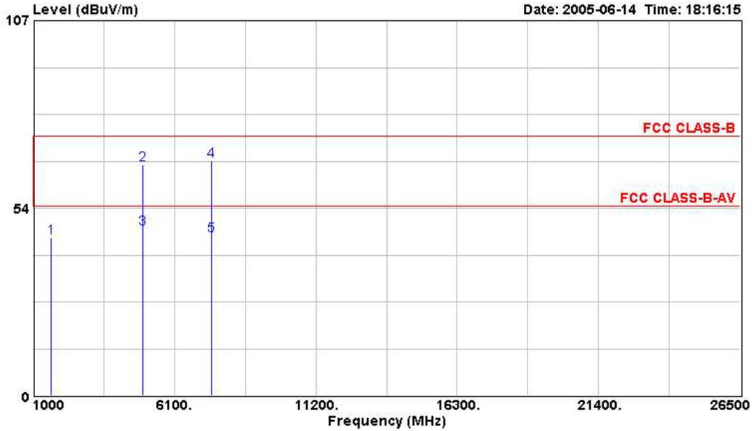
Table 1: Emission Levels (dBuV/m) vs Frequency (MHz)
