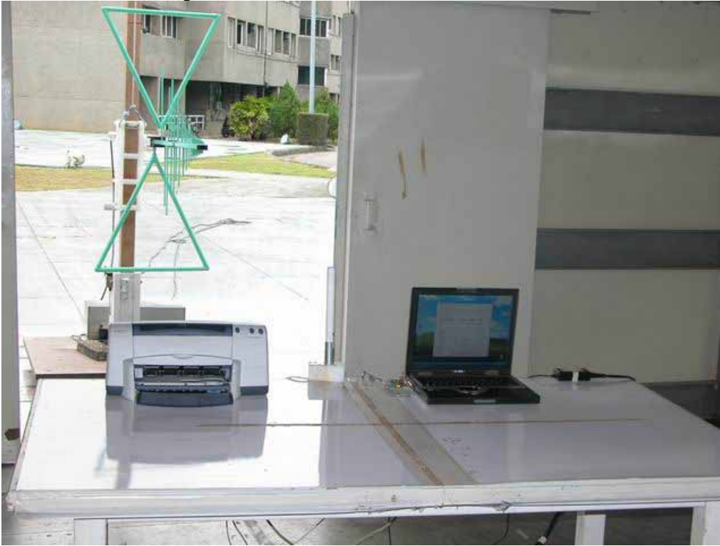
Antenna 3 : Antenna gain is 5dBi
