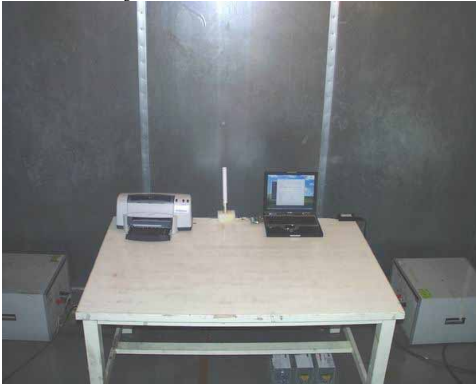
Antenna 3 : Antenna gain is 5dBi
