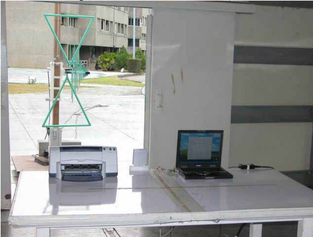
Antenna 6 : Antenna gain is 7.5dBi
