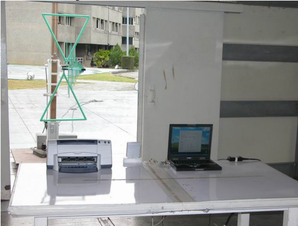
Antenna 6 : Antenna gain is 7.5dBi
