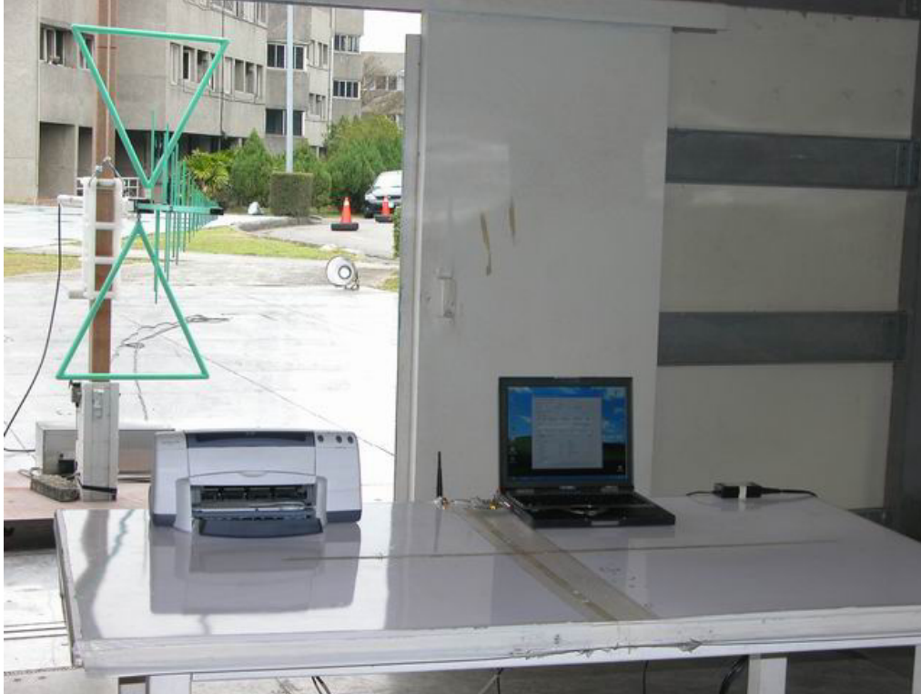
Antenna 2 : Antenna gain is 2dBi
