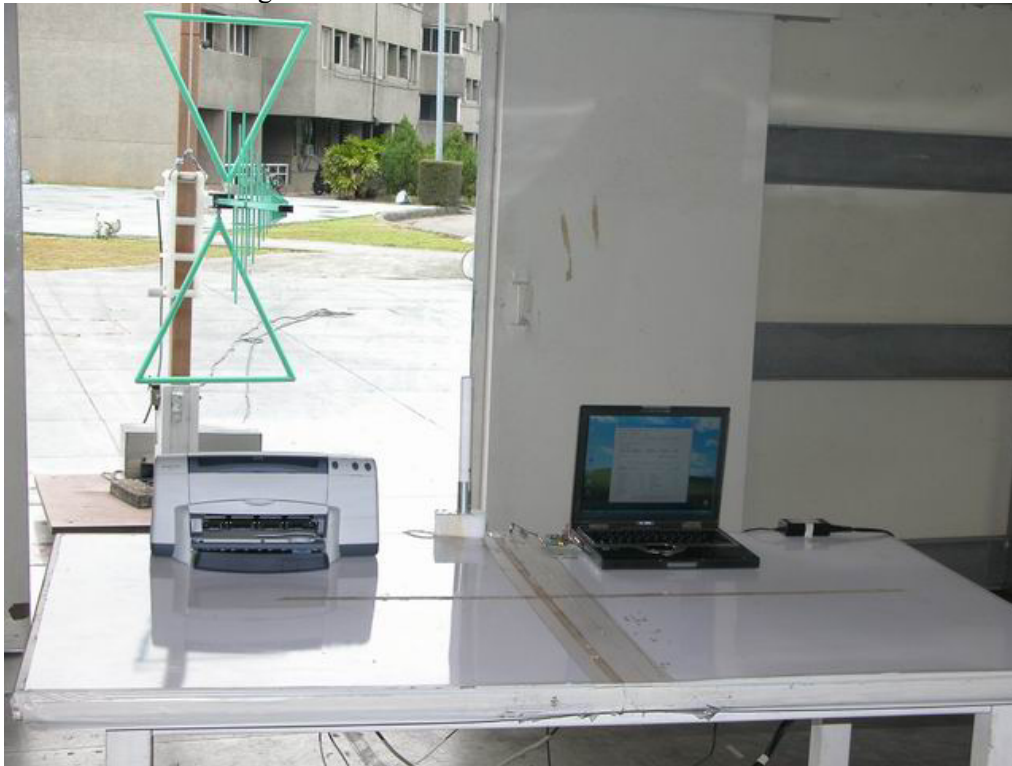
Antenna 3 : Antenna gain is 5dBi
