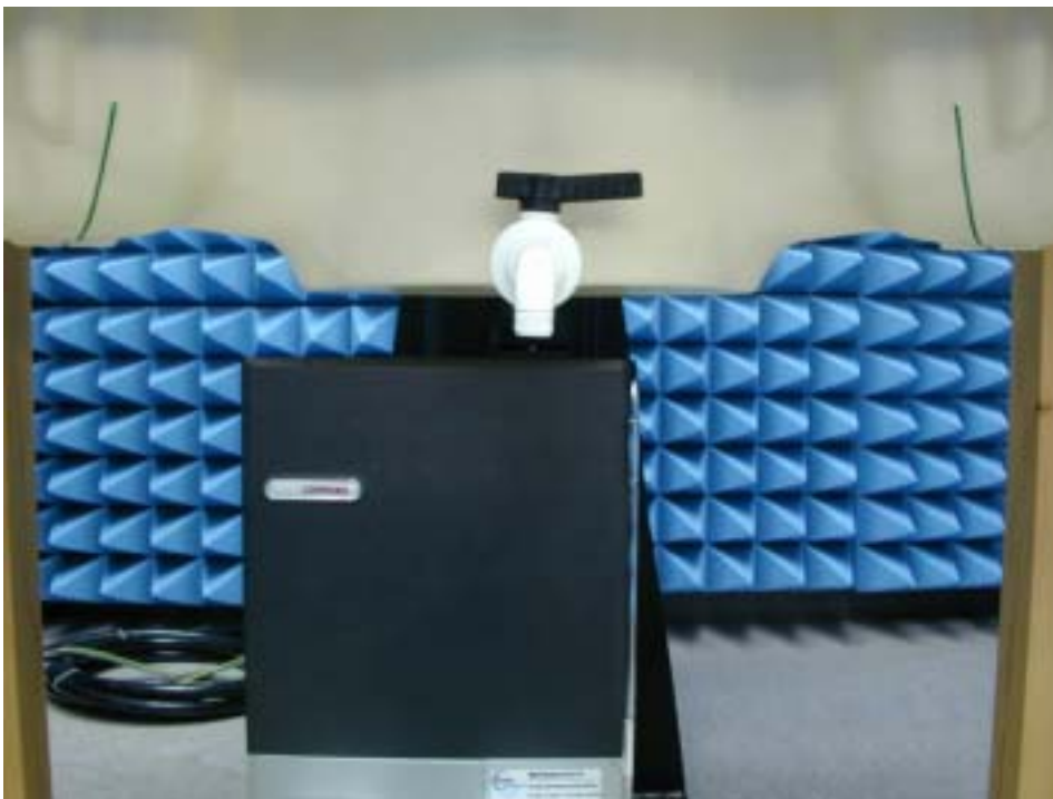
Fig.3 Photograph of the edge of the PC at 90° and at a distance of 1.5 cm from the base of the phantom
