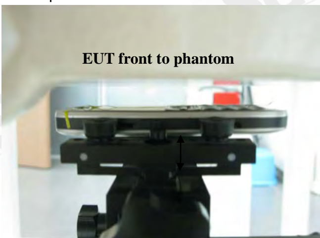
Fig.8 Body worn- EUT front to flat phantom and distance between flat phantom and mobile phone is 1.5 cm
