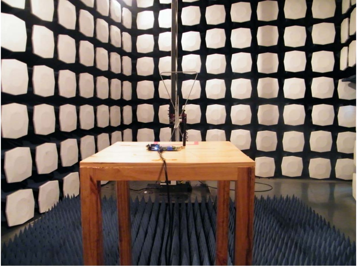
Picture 2: Radiated Spurious Emissions Test setup
