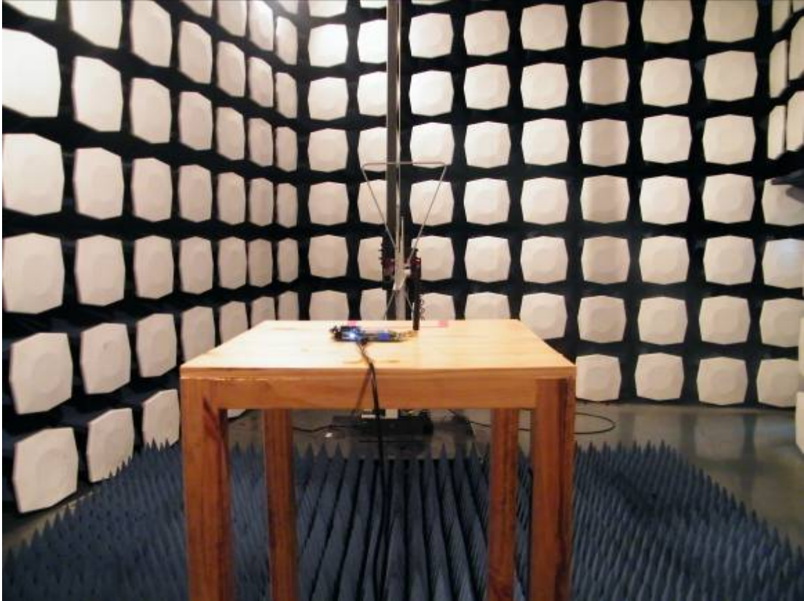
Picture 2: Radiated Spurious Emissions Test setup
