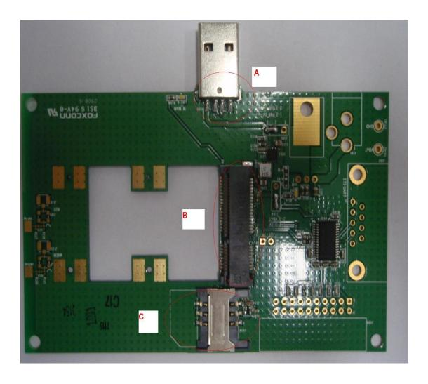
A: USB port B: MV82P1 card socket C: SIM card socket
