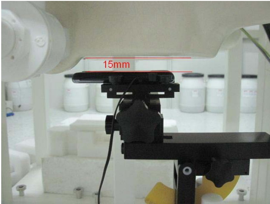
Body SAR Back 15mm with Headset
