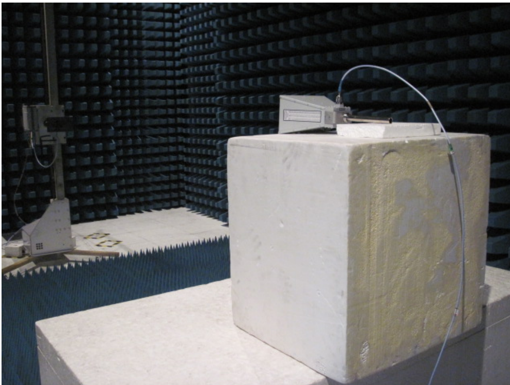
Description: Substitution Antenna for EIRP Test
