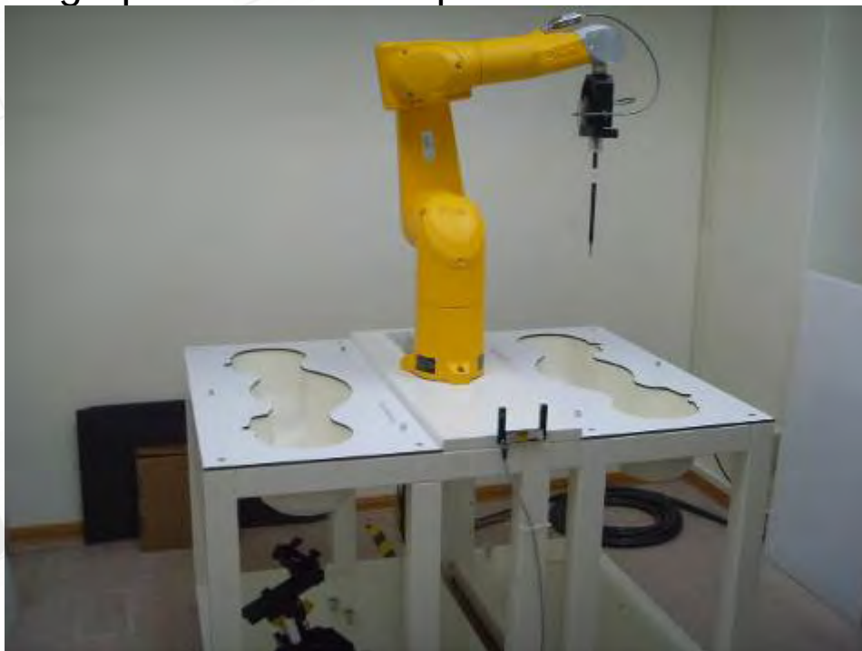
Fig.1 Photograph of the SAR measurement System
