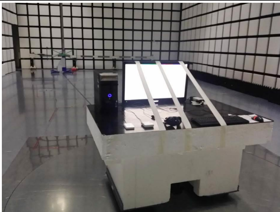
Figure 3. Radiated Emission Test Setup (30 MHz ~ 1 GHz) : DVI Mode
