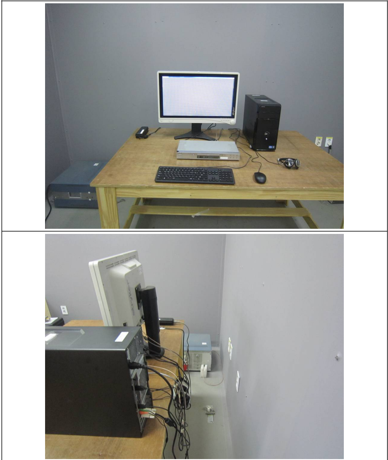
Figure 1. Conducted Emission Test Setup : DVI Mode
