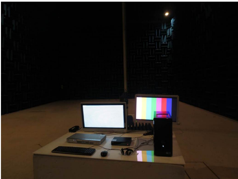
Figure 6. Radiated Emission Test Setup (1 ~ 6) GHz : SDI In-Out Mode
