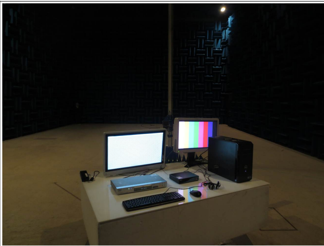
Figure 4. Radiated Emission Test Setup (1 ~ 6) GHz : DVI Mode
