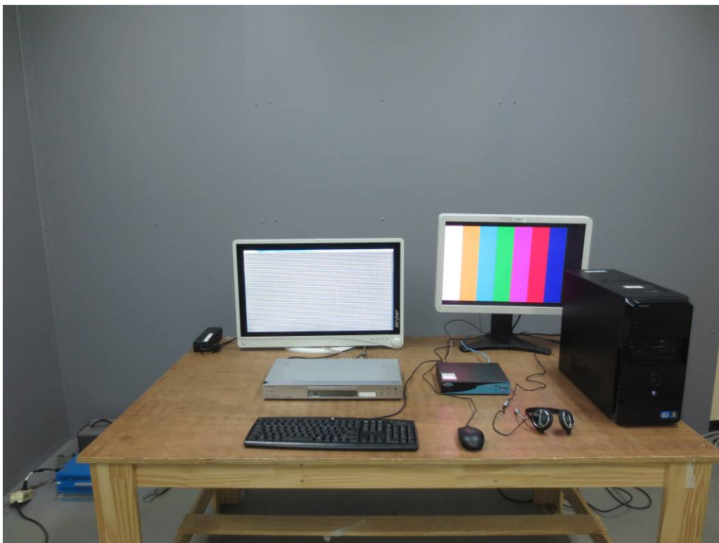
Figure 1. Conducted Emission Test Setup : DVI Mode
