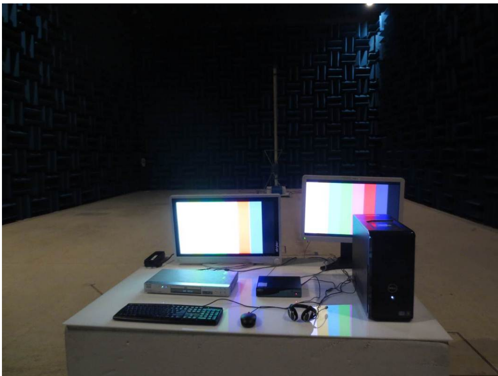
Figure 5. Radiated Emission Test Setup (30 MHz ~ 1 GHz) : SDI In-Out Mode
