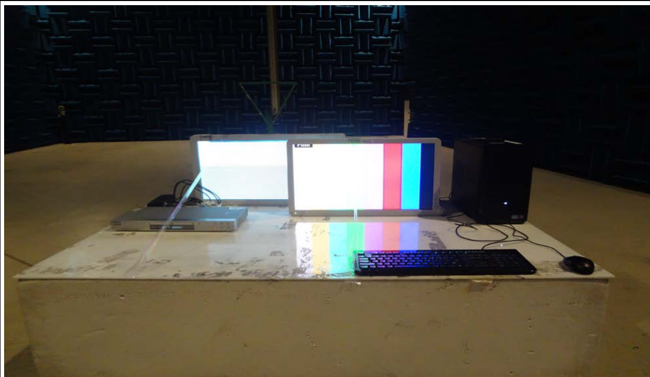
Figure 3. Radiated Emission Test Setup (30 MHz ~ 1 GHz) : DVI Mode
