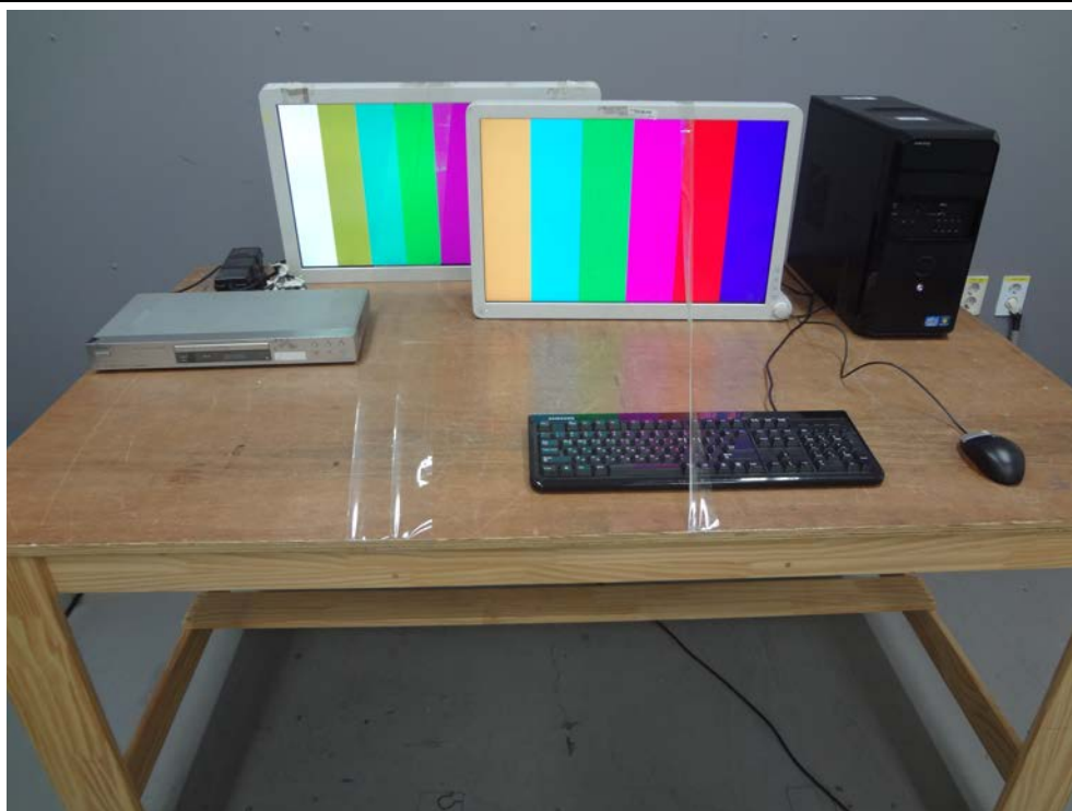
Figure 2. Conducted Emission Test Setup : SDI Mode
