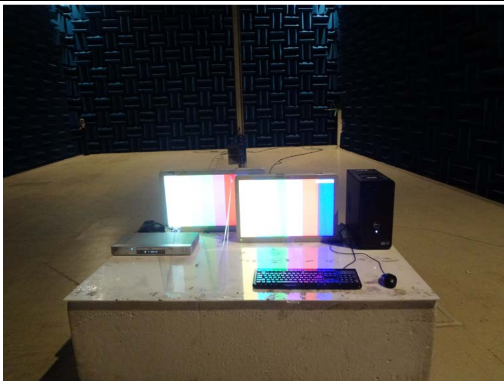
Figure 6. Radiated Emission Test Setup (1 ~ 6) GHz : SDI Mode
