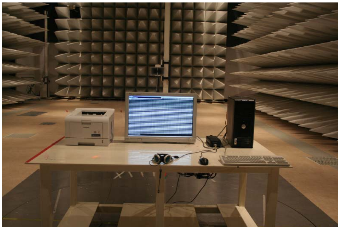
Figure 6. Photo of Radiated emission test setup for Test Configuration #1, 1GHz to 2GHz
