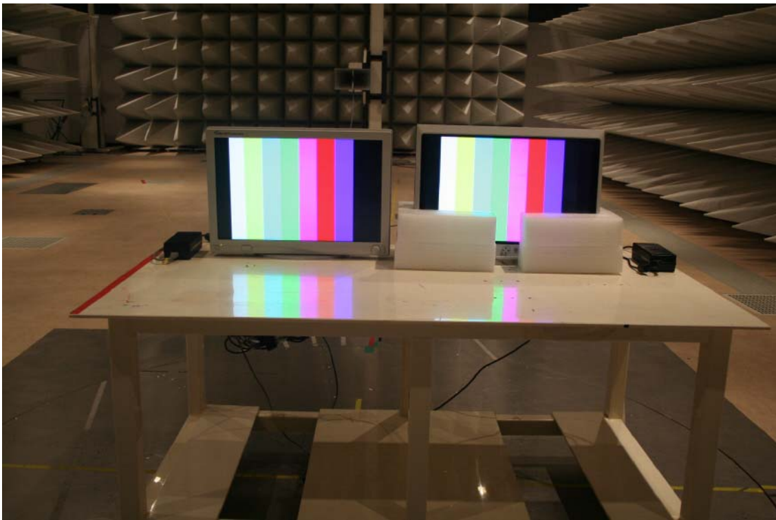
Figure 8. Photo of Radiated emission test setup for Test Configuration #1, 1GHz to 2GHz
