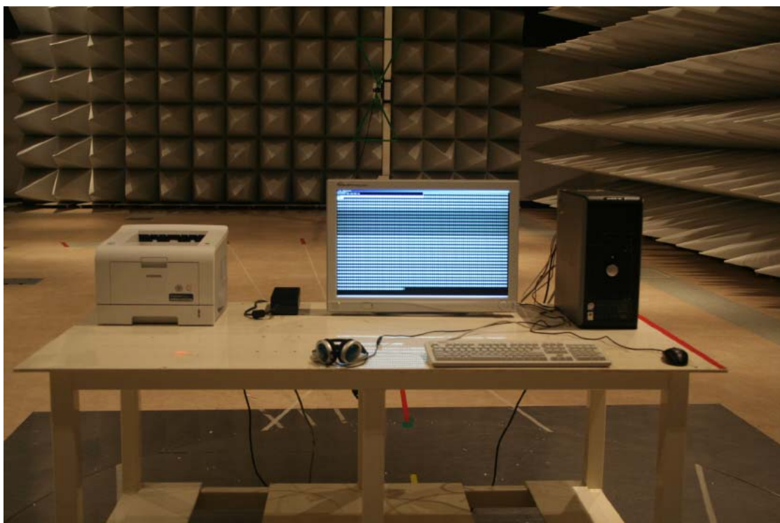
Figure 5. Photo of Radiated emission test setup for Test Configuration #1, 30MHz to 1GHz
