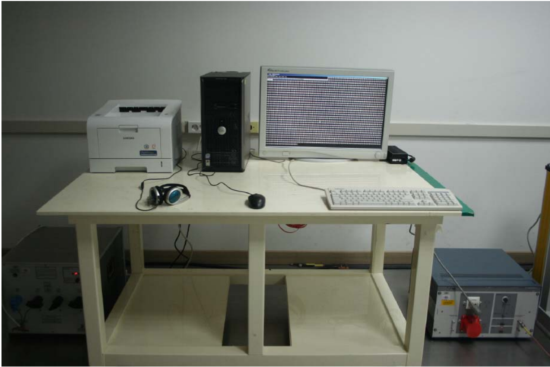
Figure 3. Conducted Emission Test Setup for Test Configuration #2
