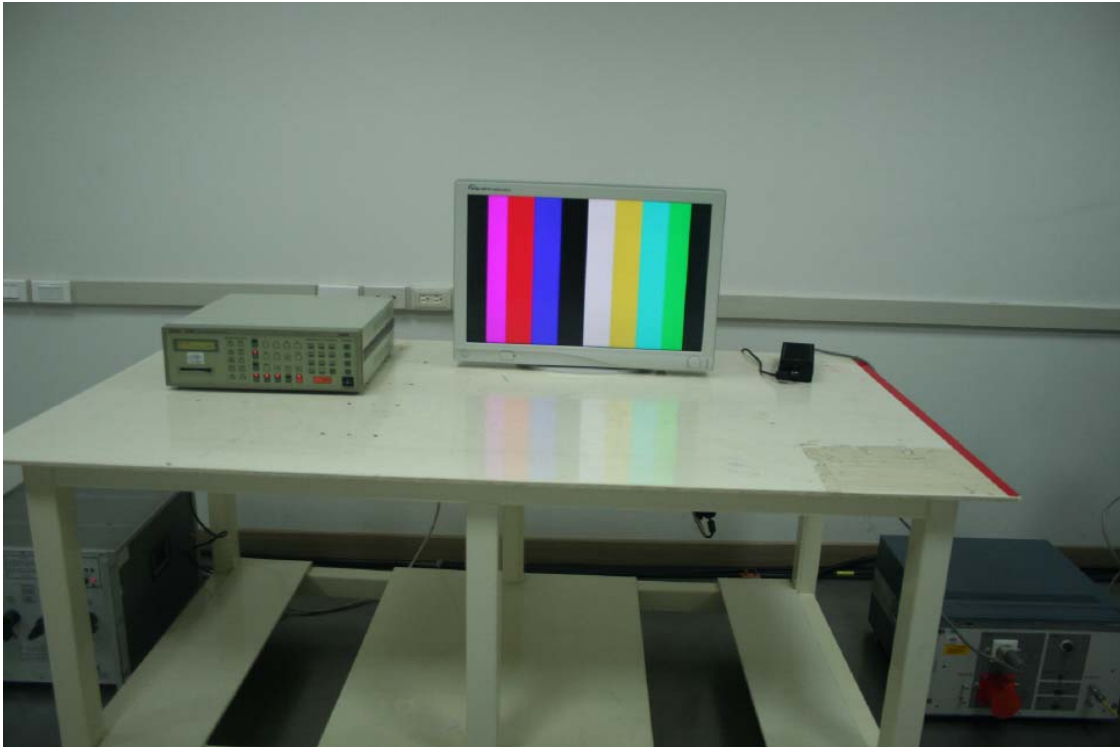
Figure 4. Conducted Emission Test Setup for Test Configuration #2
