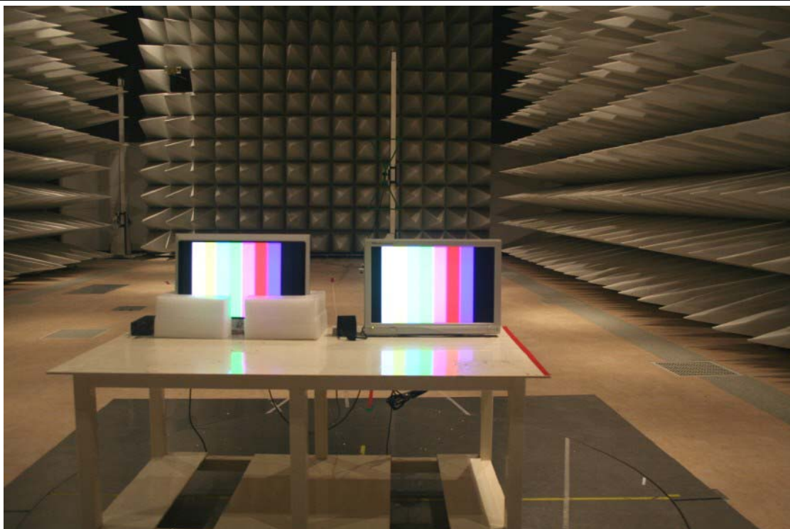
Figure 7. Photo of Radiated emission test setup for Test Configuration #1, 30MHz to 1GHz
