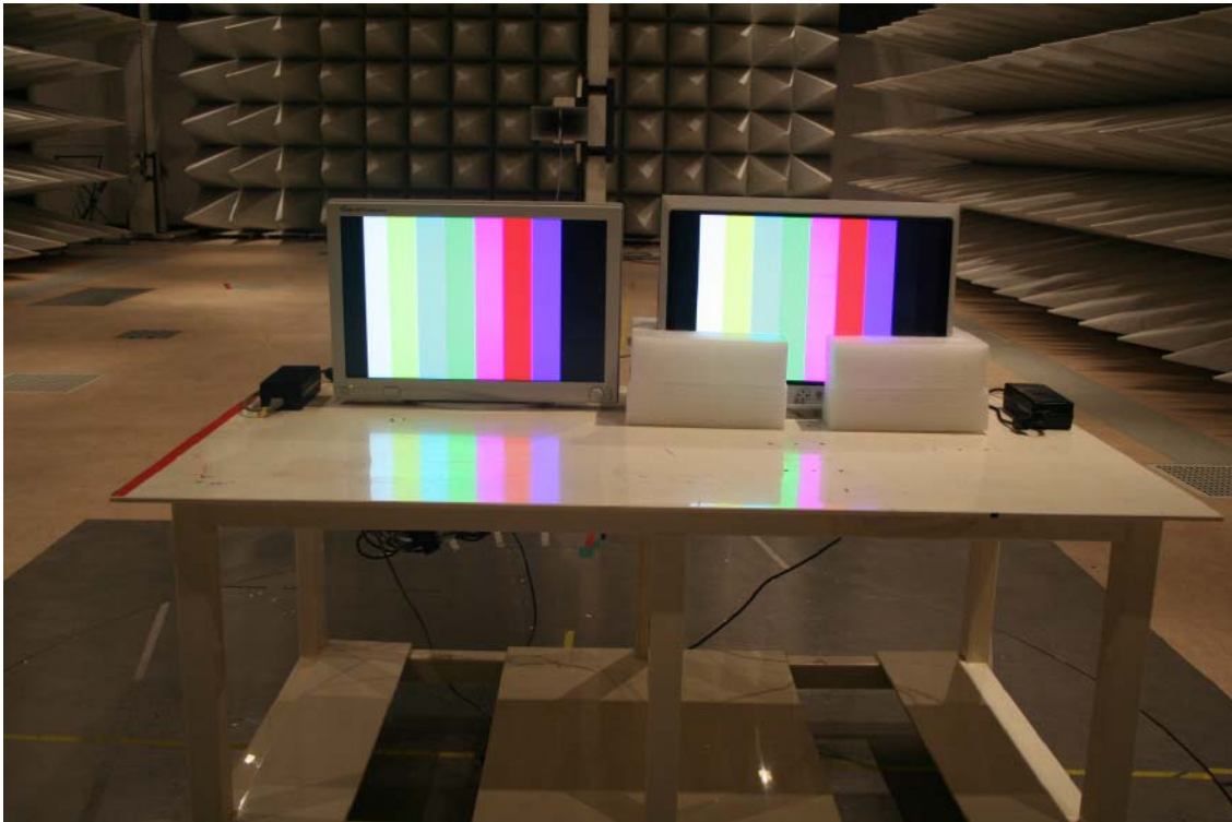
Figure 11, Photo of Radiated emission test setup of Test Mode #1, 1.0 GHz to 2.0 GHz
