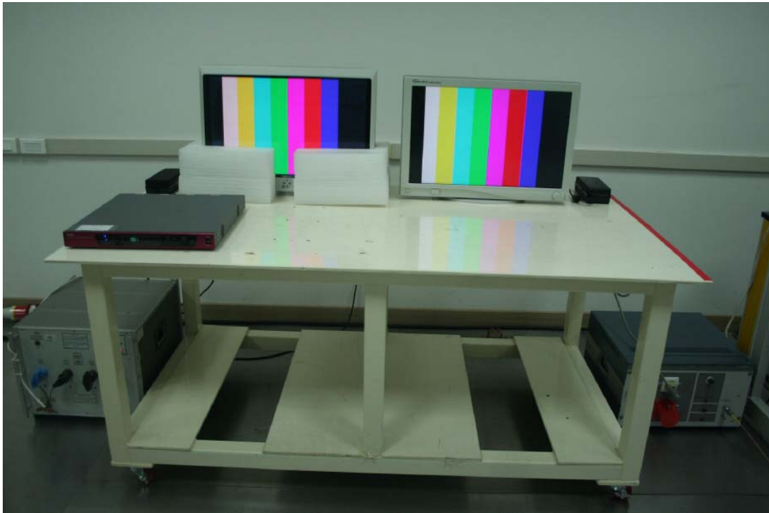
Figure 2. Conducted Emission Test Setup of Test Mode #1
