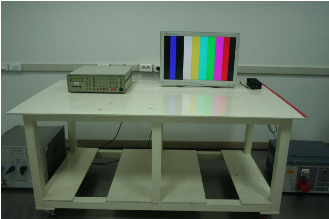
Figure 4. Conducted Emission Test Setup of Test Mode #2
