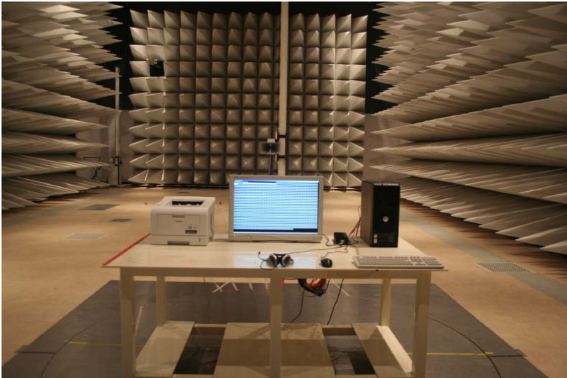
Figure 11, Photo of Radiated emission test setup of Test Mode #2, 1.0 GHz to 2.0 GHz
