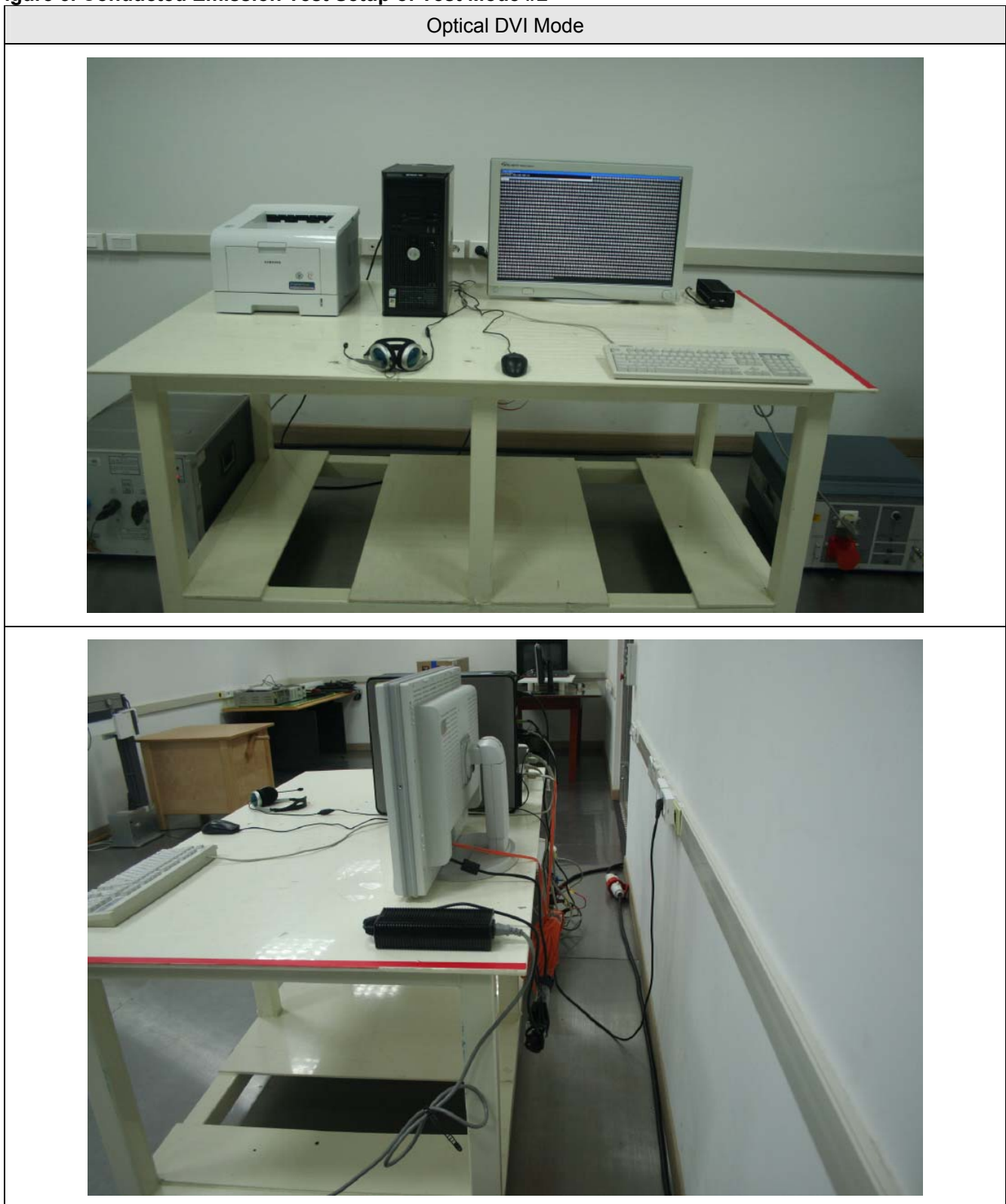
Figure 3. Conducted Emission Test Setup of Test Mode #2
