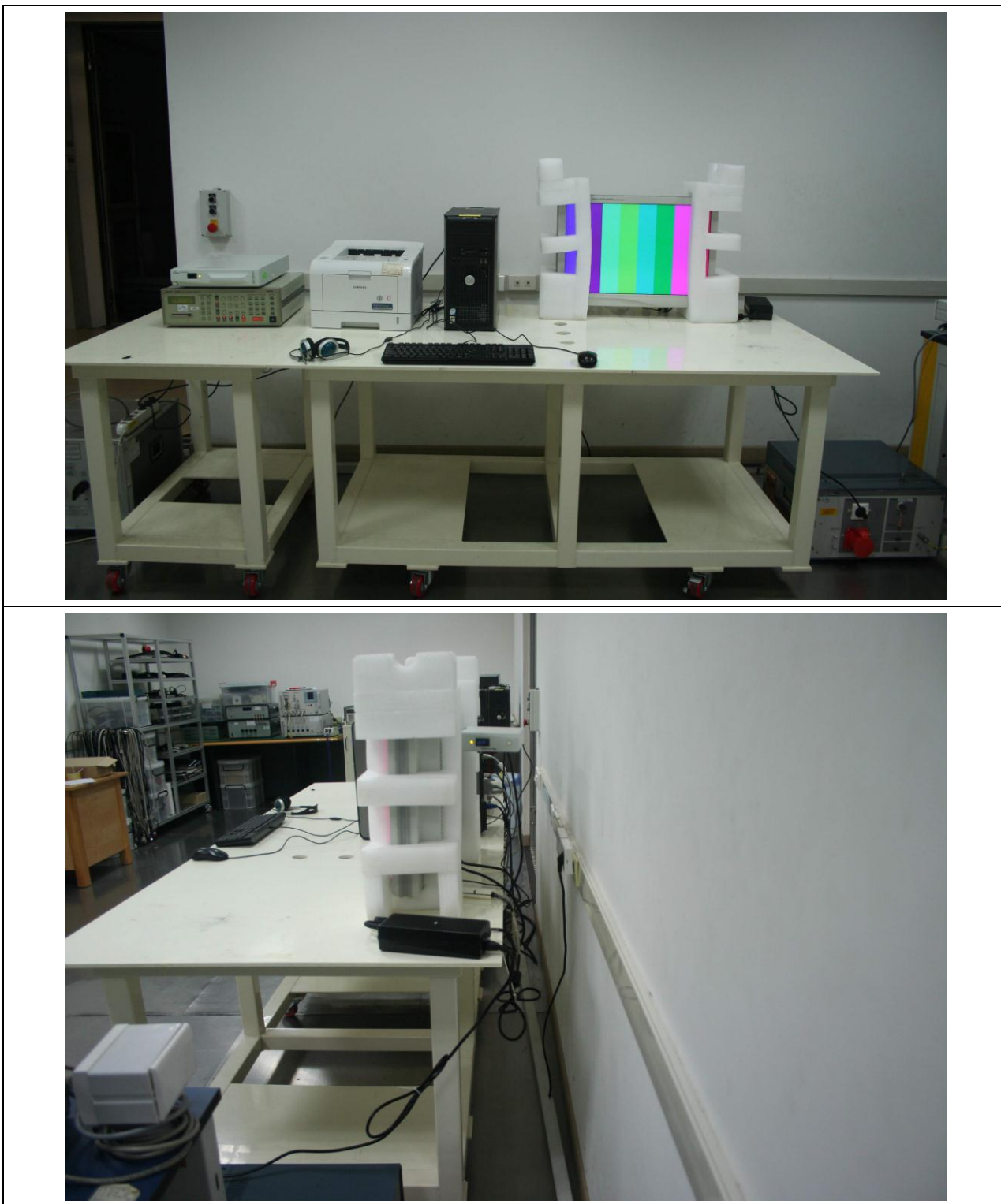
Figure 1. Conducted Emission Test Setup for Wireless RGB Mode:
