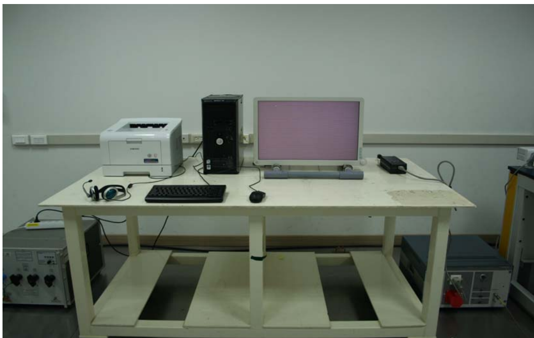
Figure 1. Conducted Emission Test Setup for Test Configuration #1
