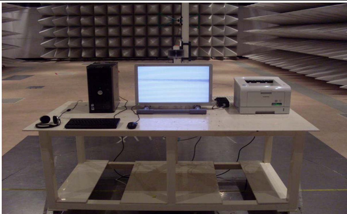
Figure 12. Photo of Radiated emission test setup for Test Configuration #2, 1GHz to 2GHz
