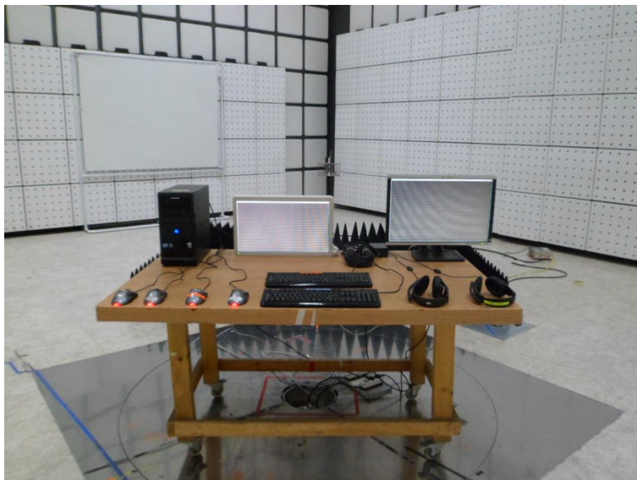
Figure 4. Radiated Emission Test Setup (1 ~ 6) GHz : PColP Mode
