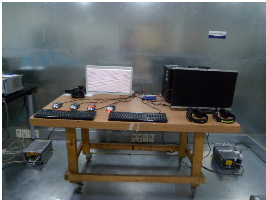
Figure 2. Conducted Emission Test Setup : VGA Mode
