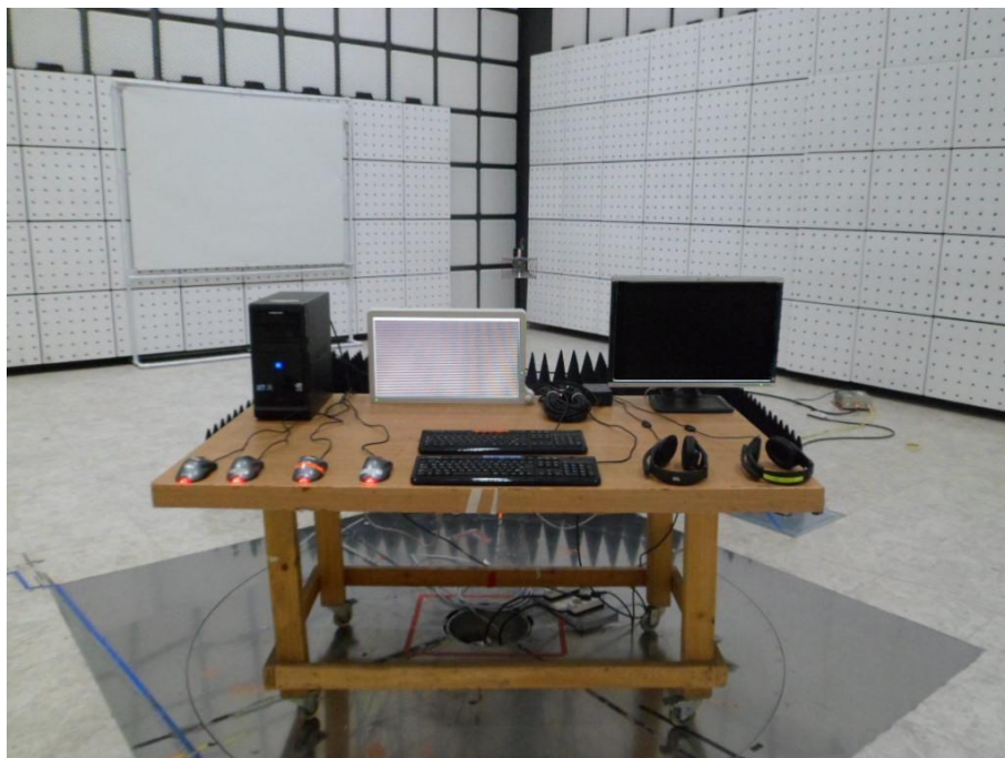
Figure 6. Radiated Emission Test Setup (1 ~ 6) GHz : VGA Mode
