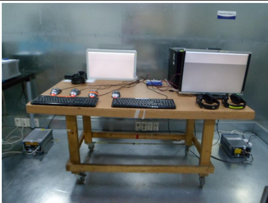
Figure 1. Conducted Emission Test Setup : PCoIP Mode
