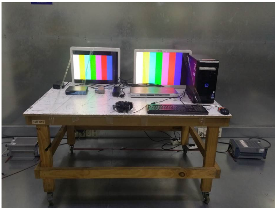
Figure 2. Conducted Emission Test Setup : SDI Mode
