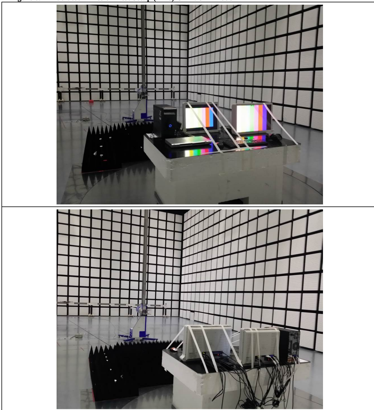
Figure 6. Radiated Emission Test Setup (1 ~ 6) GHz : SDI Mode
