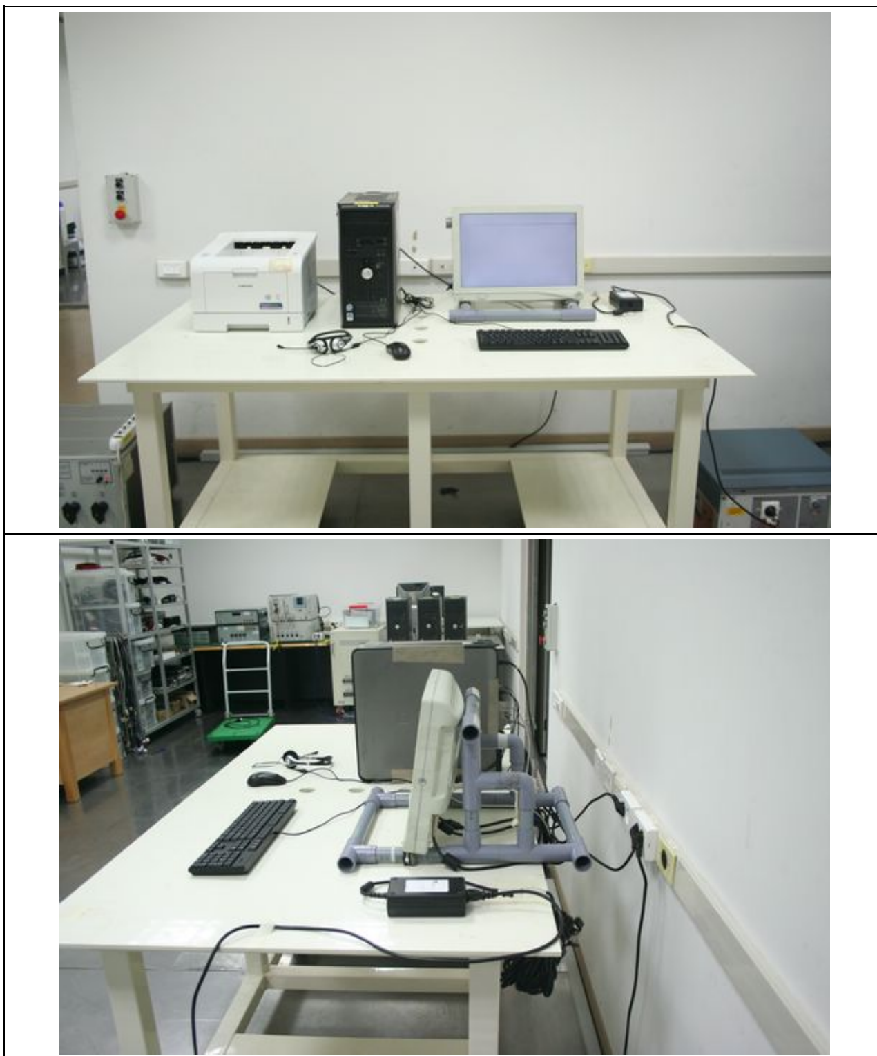
Figure 1. Conducted Emission Test Setup for DVI Mode:
