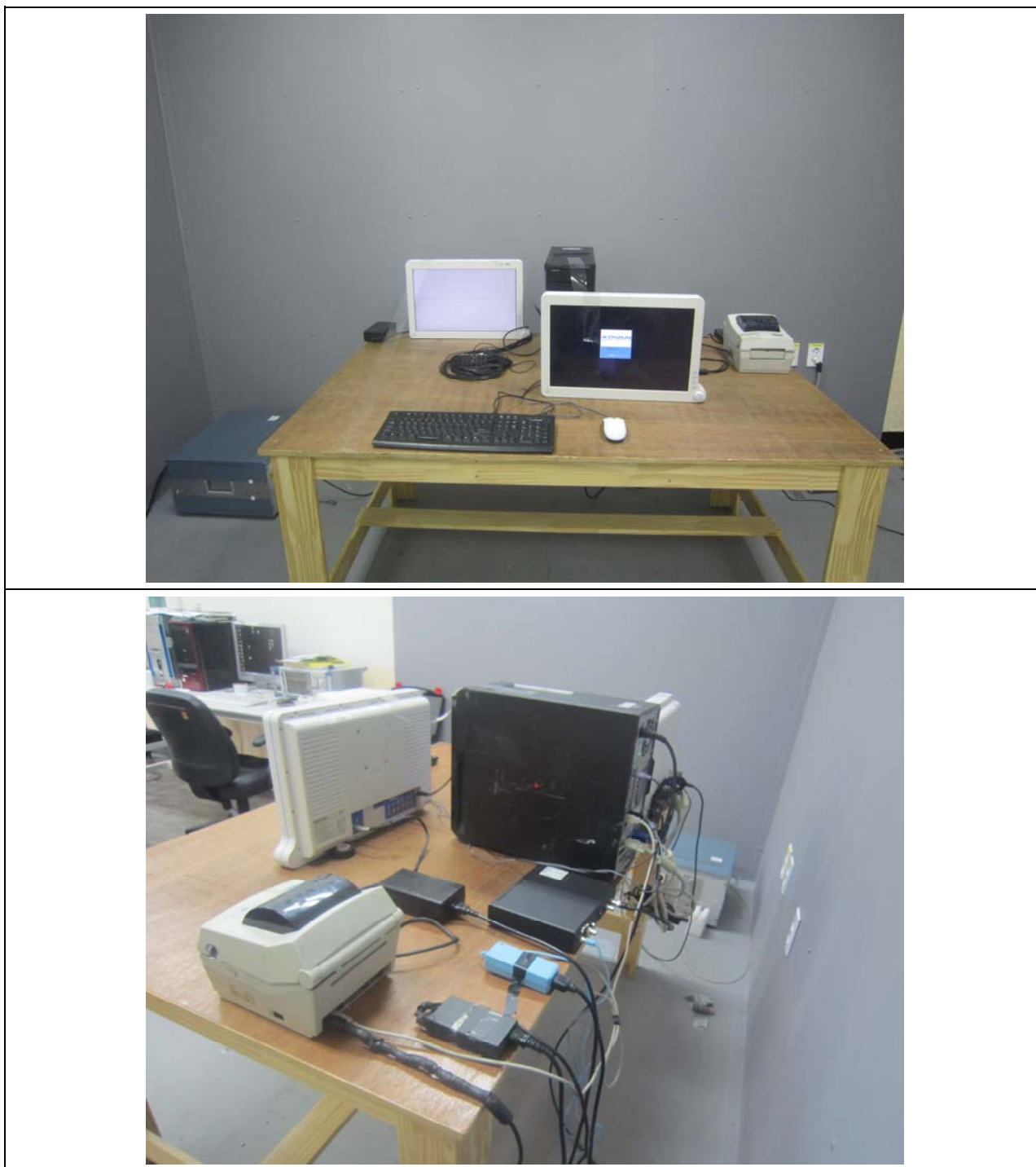
Figure 1. Conducted Emission Test Setup: DSUB Mode
