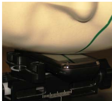
Photo of the device in “cheek” position
