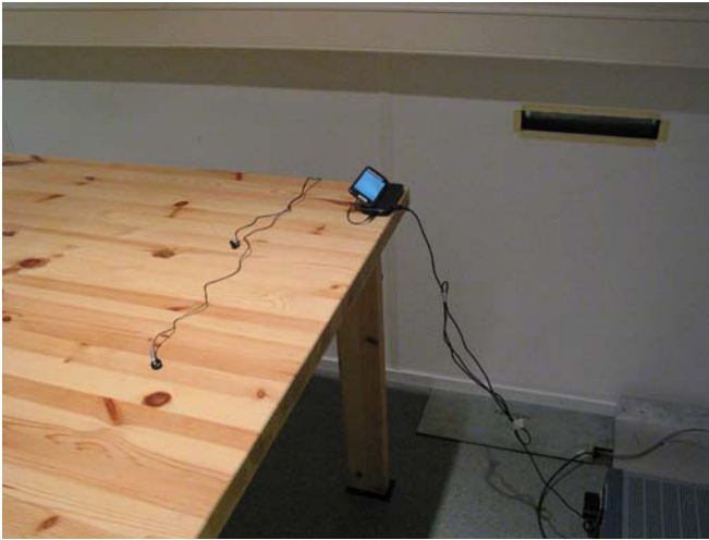
Picture 3 AC powerline conducted emission measurement 15C
