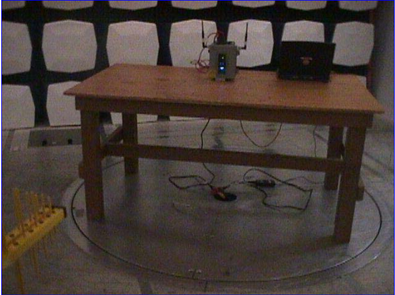
Photograph 2. Radiated Emission Limits, Test Setup
